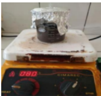
Figure 1. Rice husk ash stirring process with distilled water
