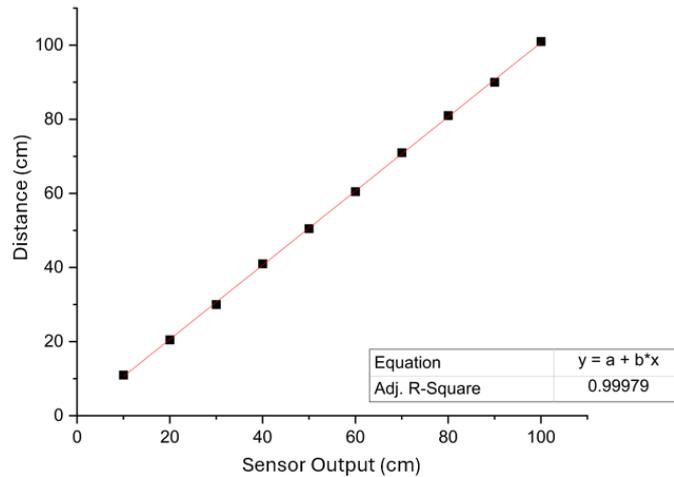
Figure 5. Ultrasonic Sensor Characteristics
