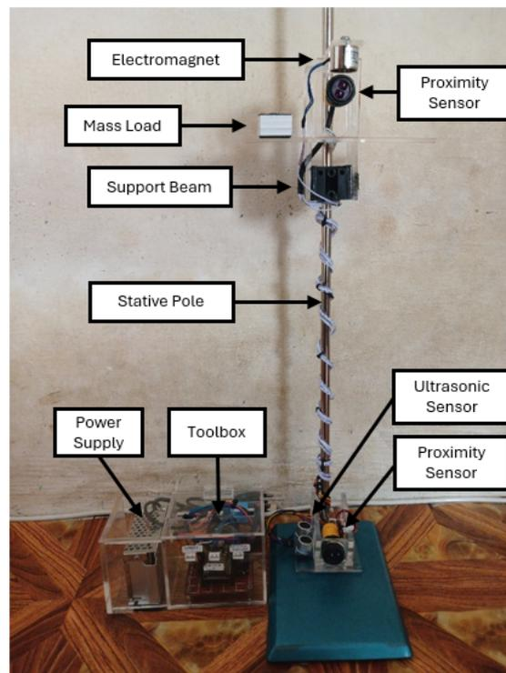
Figure 7. System Mechanics
