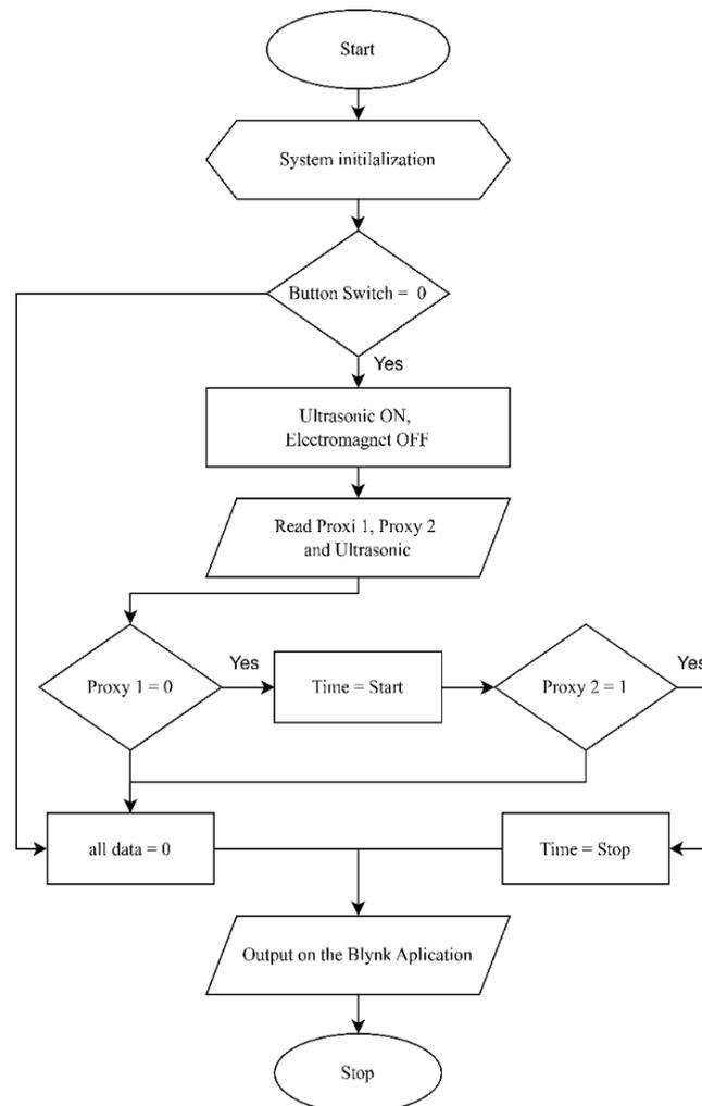
Figure 3. Software design / flowchart
