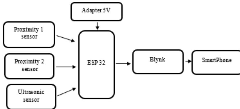
Figure 1. Tool Block Diagram
