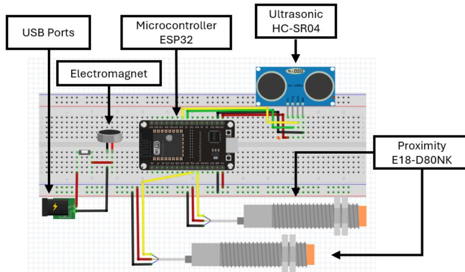
Figure 4. Electronic Circuit System
