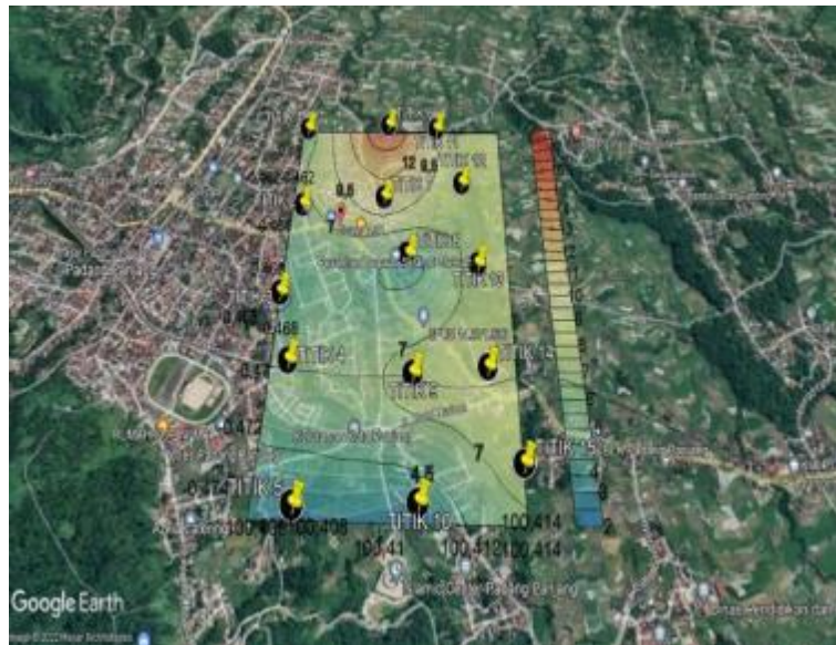
Figure 5. Map of The Distribution of Dominant Frequency Values Overlaid With Google Earth
