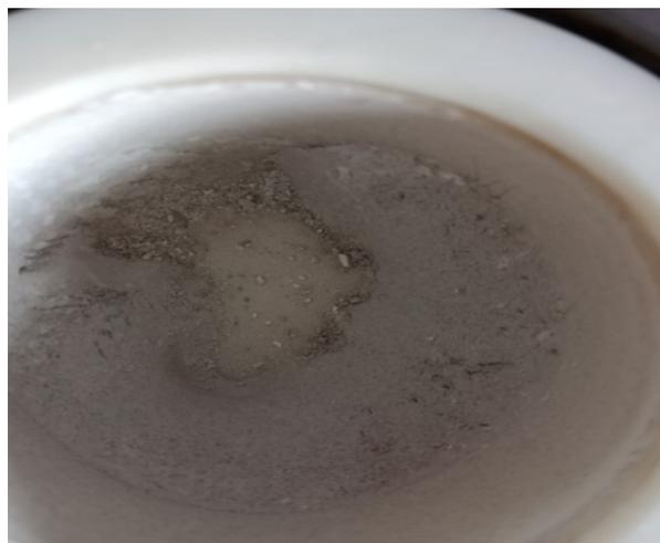
Figure 4. Coconut husk ash after milling
