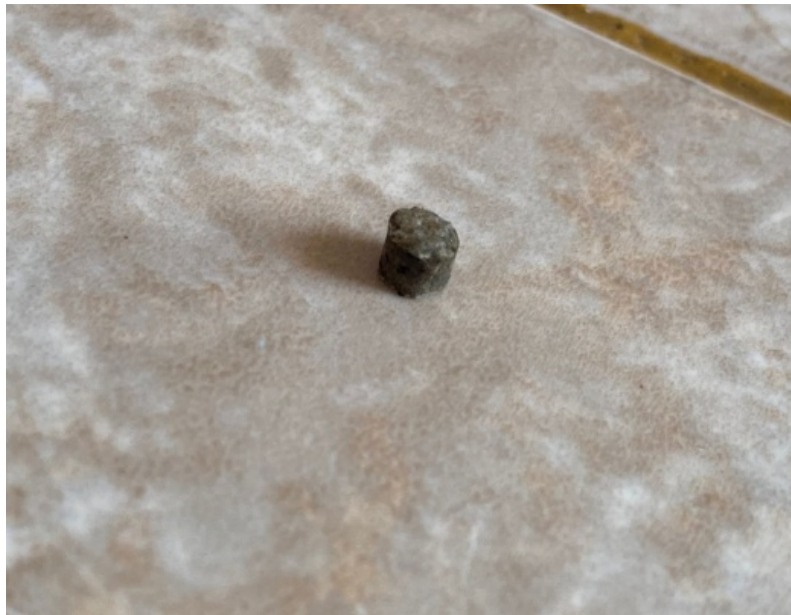
Figure 5. The shape of the pellets from zeolite before the LCR meter is carried out
