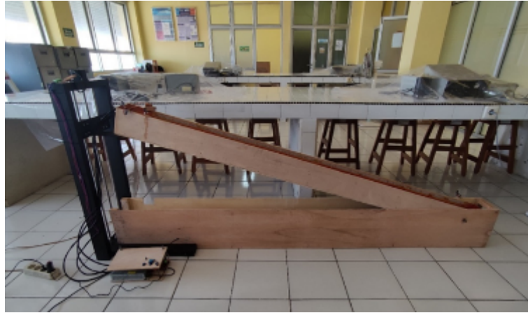
Figure 3. The outcome hardware design of Translation Motion in Constant Acceleration experiment instrument
