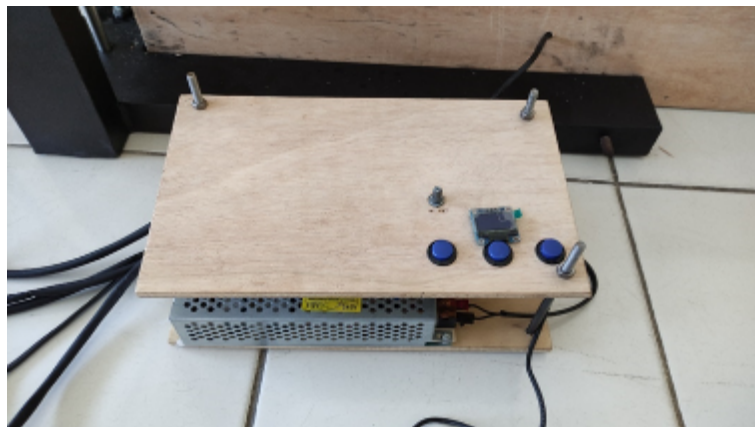
Figure 4. Circuit box of Translation Motion in Constant Acceleration experiment instrument
