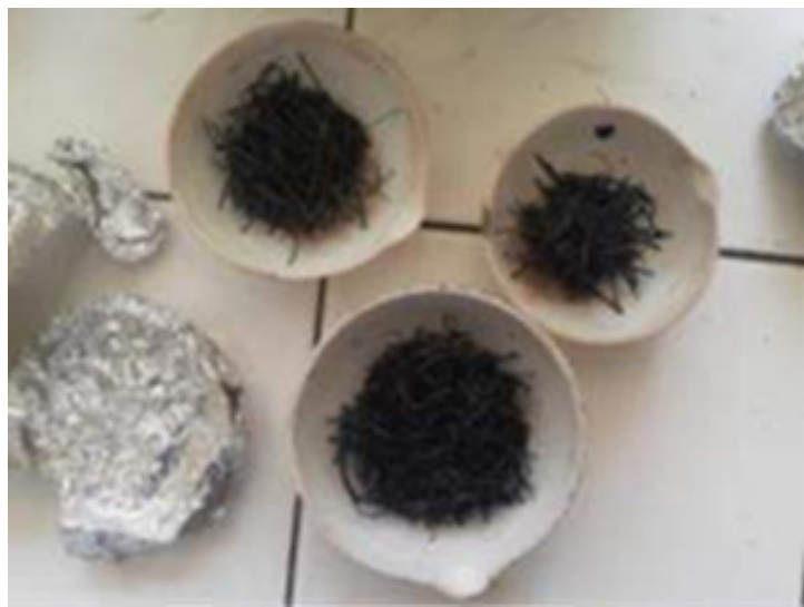
Figure 1. Charred bamboo from a furnace
