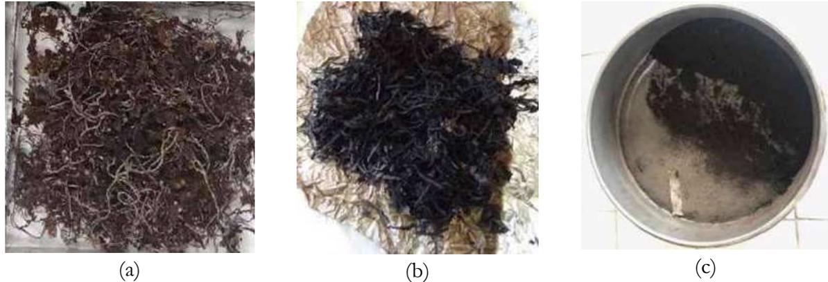
Figure 1. Sample Preparation (a) Drying (b) Carbonization (c) Sifting
