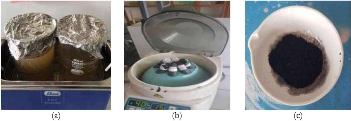
Figure 4. GO Dispersion Process (1) Sonication (2) Centrifugation (3) GO Powder
