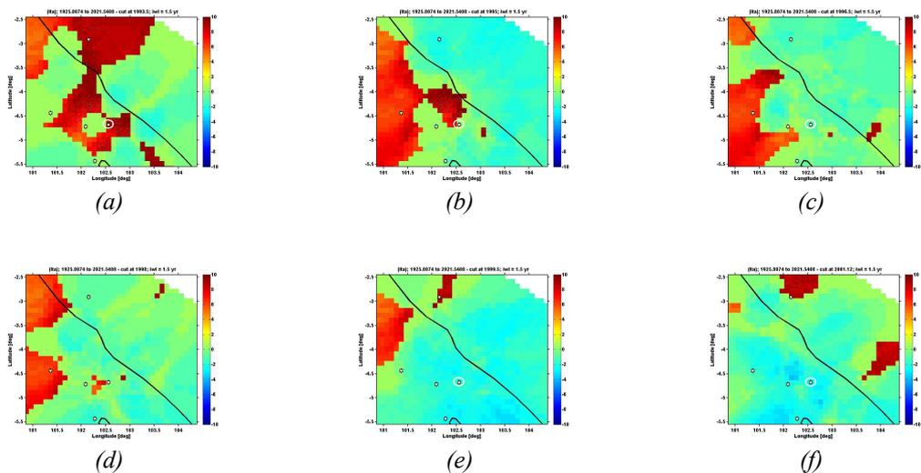
Figure 7. The spatial distribution of z-values before the 2001 earthquake event (7.0 on the Richter scale) with an iwl of 1.5 years (a) cut at 1993.5 (b) cut at 1995 (c) cut at 1996.5 (d) cut at 1998 (e) cut at 1999.5 (f) cut at 2001.12.
