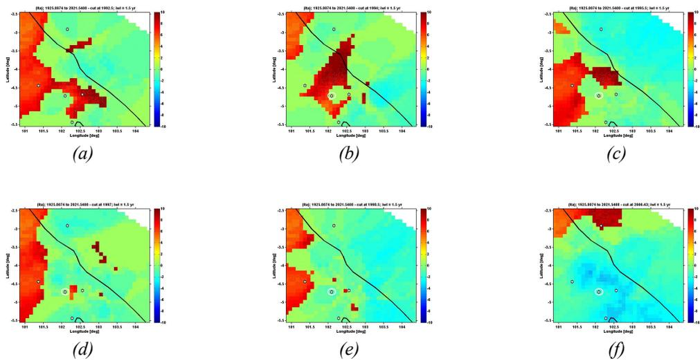
Figure 6. The z-value's spatial distribution prior to the 2000 earthquake event (7.0 on the Richter scale) with an iwl of 1.5 years (a) cut at 1992.5 (b) cut at 1994 (c) cut at 1995.5 (d) cut at 1997 (e) cut at 1998.5 (f) cut at 2000.43
