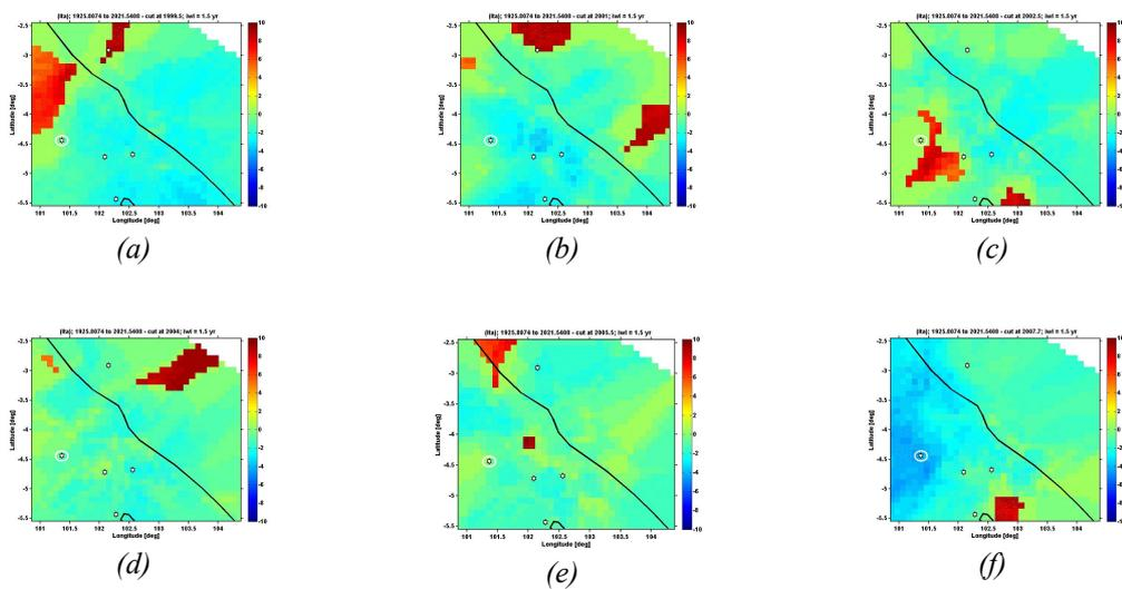
Figure 8. The spatial distribution of z-value before the 2007 earthquake event (7.7 SR) with an iwl of 1.5 years (a) cut at 1999.5 (b) cut at 2001 (c) cut at 2002.5 (d) cut at 2004 (e) cut at 2005.5 (f) cut at 2007.7.
