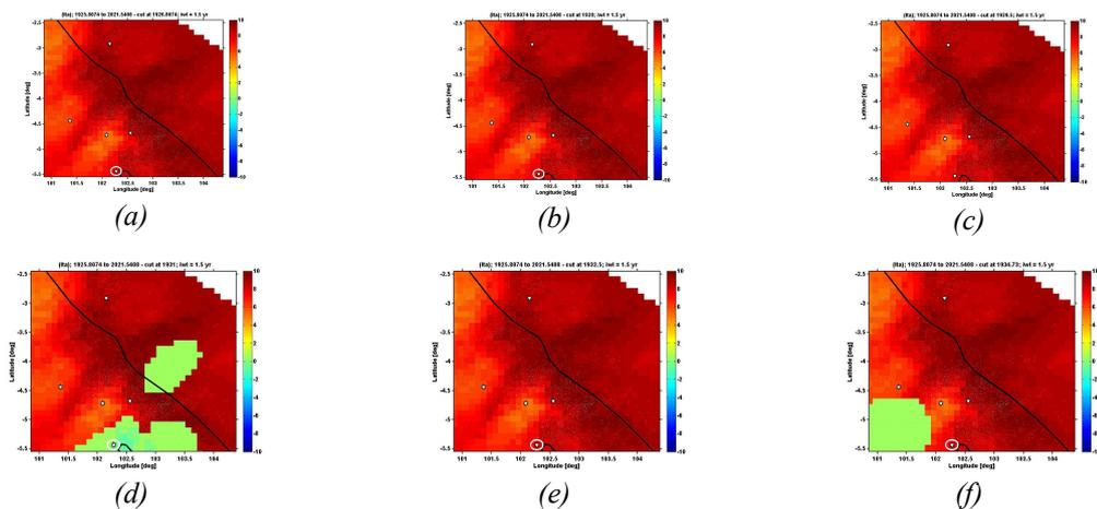
Figure 4. The z-value's spatial distribution prior to the 1934 earthquake event (7.0 SR) with  $iwl = 1.5$  years: (a) cut at 1926.5 (b) cut at 1928 (c) cut at 1929.5 (d) cut at 1931 (e) cut at 1932.5 (f) cut at 1934.73
