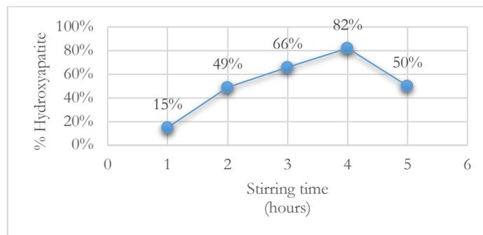
Figure 3. Stirring Time vs Hydroxyapatite Percentage
